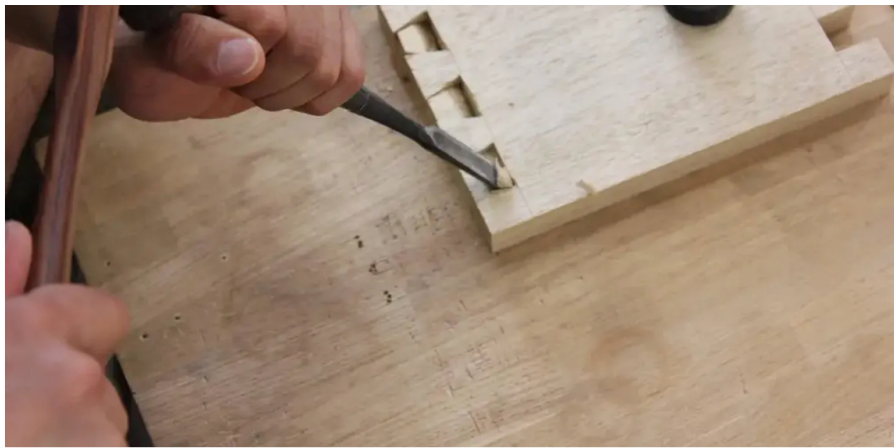
Maker Masahiro Kudo making a mortice joint. Photo courtesy of Japan Woodcraft Association
